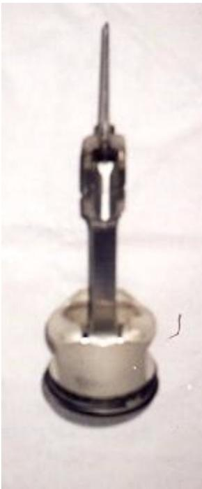
The next important component is the connecting rod. Don Vogt (a highly respected engine builder) turned me on to this one. Kohler made an 18 hp version of the K341, which they called the K361. It was a K341 with overhead valves. But the con rod used in this engine is an Alcoa aluminum FORGING instead of the standard die-cast part. Best of all, this lovely rod fits right into the other engines perfectly. It has the same external dimensions, center distances, and mass as the die-cast rod.
