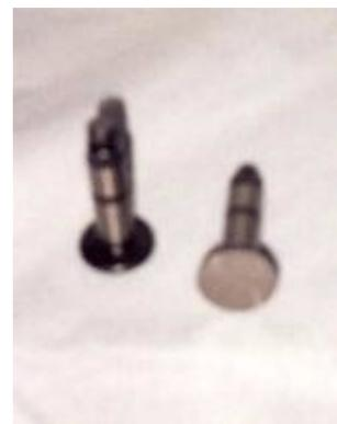
After assembly, I found that the lifters were too long and held the valves off the seats slightly. I had to surface-grind down the adjusting screws approximately .060 to allow ample clearance.
