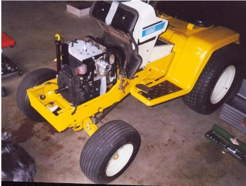
Those with sharp eyes will notice I'm using a Walbro carburetor. I discovered that these carbs can be recalibrated to work as well as the Kohler carb. It involves removing the idle calibration pocket welch plug and drilling out the progression hole using a .030 diameter drill in a pin vise. The welch plug diameter is 3/8" incidentally. The original hole diameter was .022 and thus caused that awful lean spot right off idle. I'm amazed that the as-supplied calibration was so far off.
